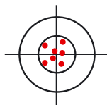
Figure 5.12 Throwing darts at the bullseye of a dartboard illustrates the notions of precision and bias. Reliable players throw precisely and without bias so that their darts hit the centre of the board accurately.
